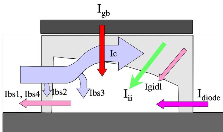
Fig. 3.1 Various current components inside the body.
