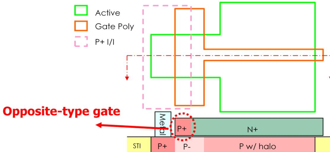
Fig. 4.4 Parasitic capacitance in opposite-type gate.
