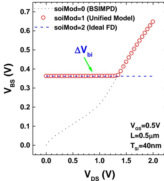
Fig. 6.1 The body potential in the unified model approaches the  $V_{BS}$  solved in BSIMPDP for PD devices, while returns to  $\Delta V_{bi}$  for ideal FD devices [20].
