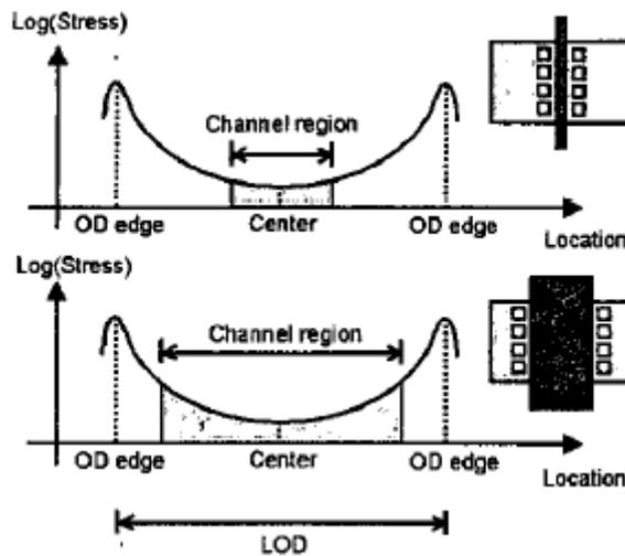
Fig. 9.2 Schematic stress distribution in the OD region [29]
