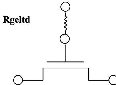
In this case, only the electrode gate resistance (bias-independent) is generated by adding an internal gate node. The electrode gate resistance  $R_{geltd}$  is given by
