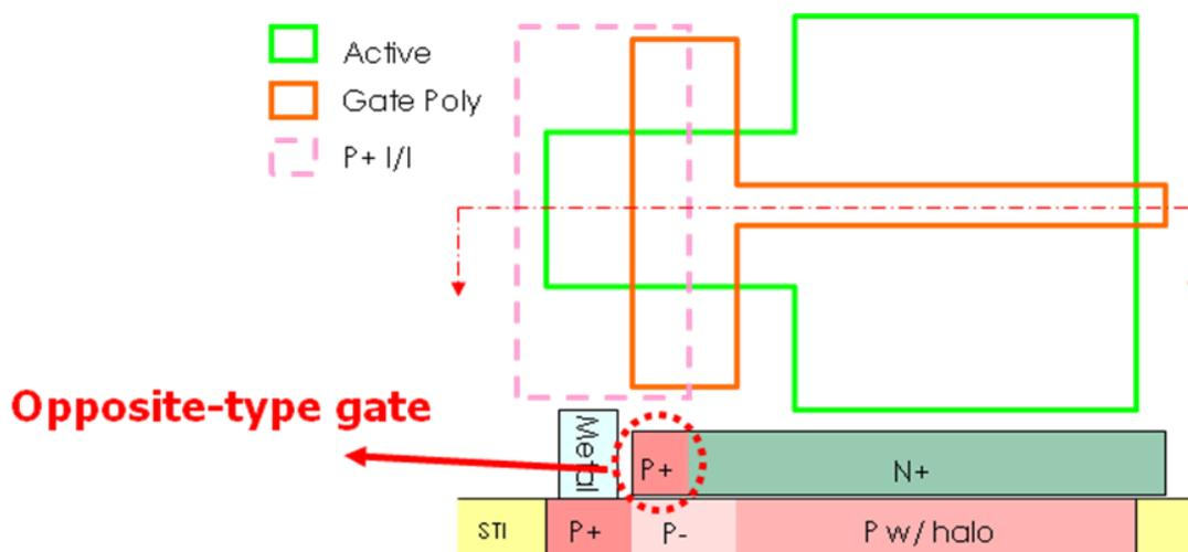
Fig. 4.4 Parasitic capacitance in opposite-type gate.
