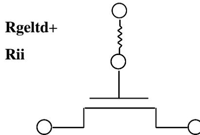
In this case, the gate resistance is the sum of the electrode gate resistance and the intrinsic-input
