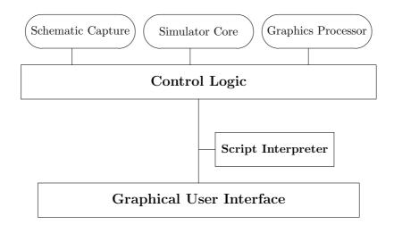
Figure 1.1: Block diagram of the *WRspice* interactive circuit simulation tool.
