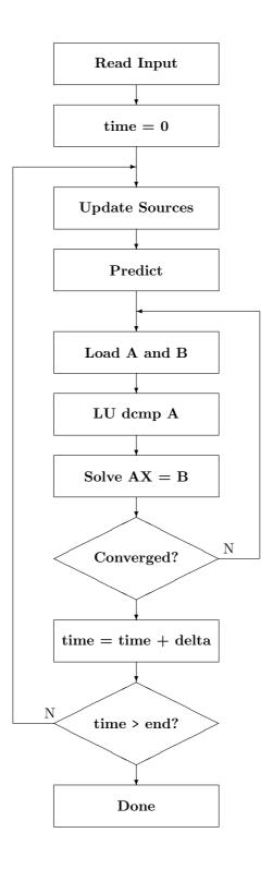
Figure 1.2: Flow diagram of the algorithm used by *WRspice*.
